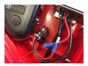
7. Repeat the crimping on the end of the bare end of the RED wire coming from the controller using the FEMALE bullet connector (the connector completely covered in blue insulation). Tug on the bullet connector to test your crimp job when done. The connectors should look like the photo to the left.
