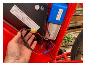
Your battery compartment should look similar to the photo at left. Tuck the cables away, close the compartment and turn ON the Sondors battery.
