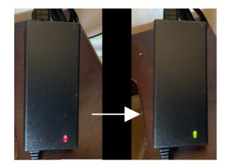
When the LED light on the AC Adapter turns from RED to GREEN the Booster Battery is fully charged.
